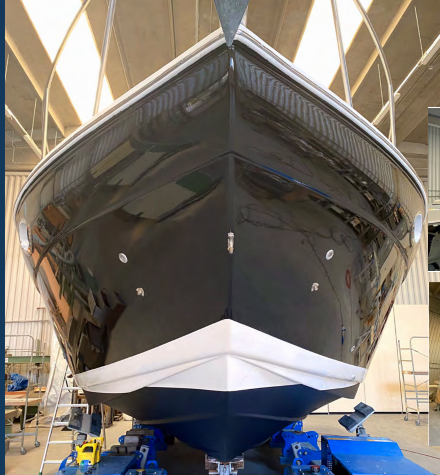
Working on Rinker 320 Painting of the hull
